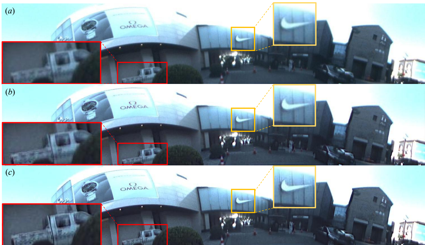
Fig. 13. Random PSFs distributions v.s. standard ones. (a) An unfolded image captured by the chosen PAL with aberration. (b) The restoration results under standard dataset. (c) The restoration results under random dataset. We Detailed patches in different FoVs are zoomed for best view.
