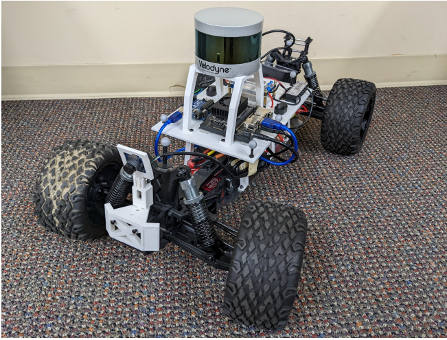
Fig. 1: Fully equipped ART 1/6th scale autonomous vehicle showing 3D printed reconfigurable mountings and support of camera, 3D lidar, and Jetson Xavier NX, the later running the autonomy stack.
