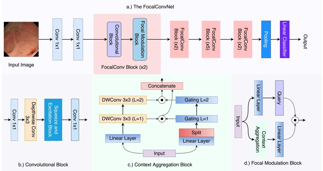
Fig. 2: **The proposed FocalConvNet architectures.** **a)** The complete FocalConvNet architecture ( $xK$  represents that the block in question has been used  $K$  times in succession), **b)** The convolutional block used with depth-wise and point-wise convolutions, **c)** Context aggregation sub-module (the figure demonstrates context aggregation when number of focal levels is 2, and can be extended in a similar manner if deeper focal levels are used), **d)** Focal modulation mechanism.
