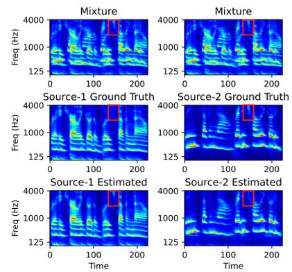
Figure 2: ConvTasnet fails to segregate fricatives in natural speech. The red boxes highlight where ‘s’ is grouped with Source-1 instead of Source-2.
