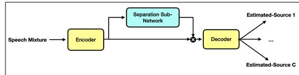
Figure 1: A typical E2E speech segregation network design
