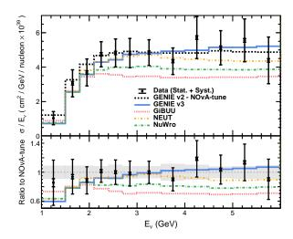
Fig. 4 Top: The differential cross section vs.  $E_{\nu}$ . Bottom: Comparisons as a ratio to the NOvA-tune prediction. The grey band represents the normalization uncertainty from the neutrino flux prediction. The data are presented showing statistical and total uncertainties.
