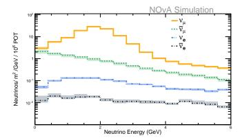
Fig. 1 NUMI neutrino-mode beam component flux spectra at the NOvA near detector below 6 GeV. The bands represent the total flux uncertainty on hadron production and beam optics for each component.
