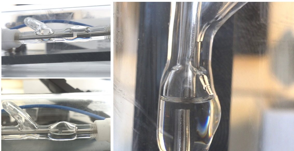
Figure 8. Experiment 5: Upper left: setup with electrodes completely covered with liquid. Lower left: reduced filling level with electrodes half covered with TMBi. Right: rotated setup with the lower electrode submerged in TMBi and the upper electrode in the gas phase. An argon pressure of 1 bar was present throughout the tests.
