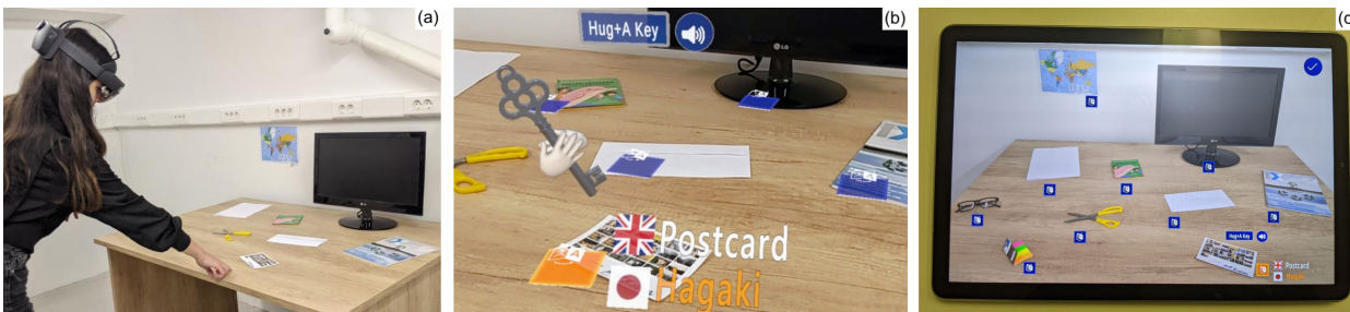
Fig. 1. VocabulARy prototype. (a) Participant interacting with VocabulARy during the study; (b) VocabulARy prototype through HoloLens2 in KEYWORD + VISUALISATION instruction mode (the Japanese word “hagaki” sounds as the English phrase “hug a key” (keyword) and visualised with an animated hand grabbing a key (visualisation)); (c) Participant interacting with non-AR version of VocabulARy in KEYWORD instruction mode (Note there is no visualisation of the keyword). AR and non-AR condition were tested with both instruction modes.
