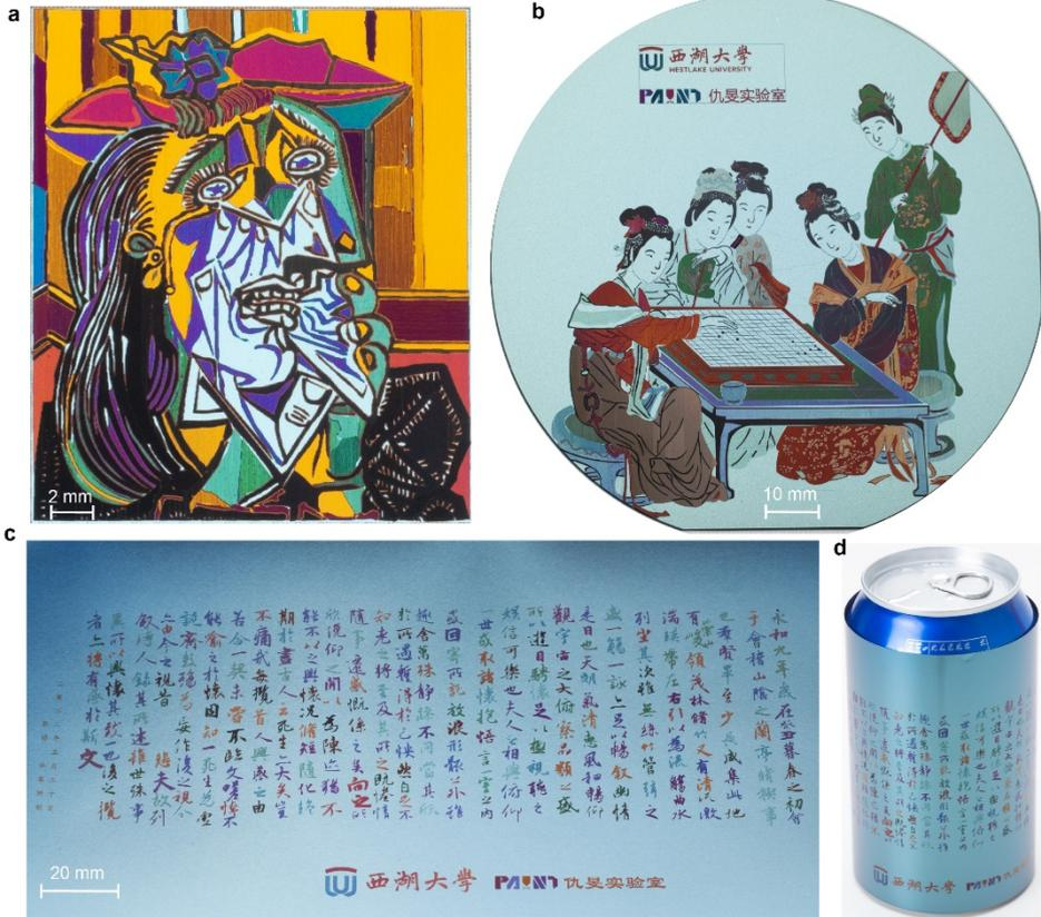
**Fig. 4 Laser coloring of large areas for painting, a-c,** Photographs of structural color- based patterns which are printed on different substrates, including polished **a**, unpolished **b** 4-inch Si wafers and large-scale stainless-steel foil **c**. The thickness of TiAlN and TiN are 60 nm and 50 nm, respectively. **d**, the same photograph in **c** while being rolled on a drink can.
