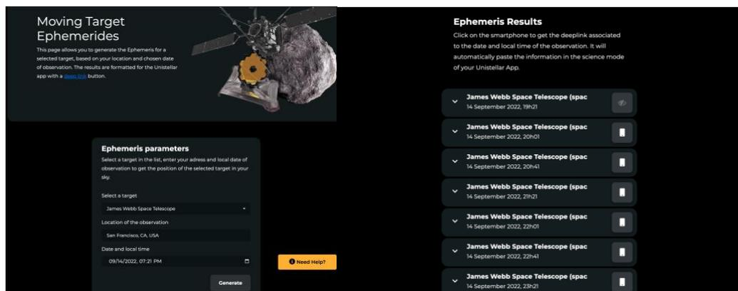
Figure 1. Ephemeris page available on the Unistellar web site (<https://unistellaroptycs.com/ephemeris/>) allowing users to generate the positions of human-made objects like JWST. The page automatically generates the position at the proper cadence for the eVscope and filters out an observation if the object is too low in elevation. A deeplink is also generated (indicated by the phone icon), which automatically opens the Unistellar App and allows the user to point their eVscope to the target.
