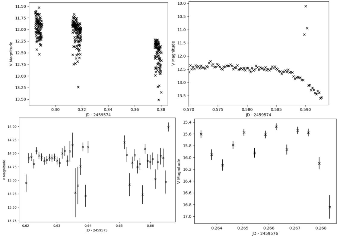
Figure 2. JWST lightcurves recorded from 2021-12-25 ~18:40 UT to 2021-12-27 18:30 UT, or 6h and 2 days after the launch, respectively. The brightness of the space telescope drops from ~12 to 16.2 magnitude. During this period of time, three Mid-Course Correction (MCC) maneuvers were applied to achieve a proper Sun-Earth/Moon L2 Libration point orbit.
