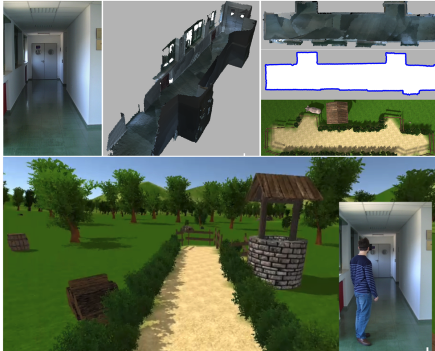
Fig. 3 The Oasis system creates a 3D map of the physical environment, automatically detecting open walkable areas which allow the system to generate virtual environments with corresponding walkable areas. While the physical affordance of walking is the same in both environments, the visual experience and spatial feel can be quite different. For example, as seen in the figure above, a hallway is transformed into an open countryside which still allows the user to walk freely while wearing a wireless headset device in the mapped physical/virtual space without breaking immersion. Figure from the paper [67].
