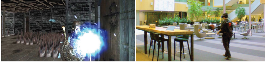
Fig. 5 VRoamer’s dungeon environment with virtual obstacles shown in response to physical obstacles in the user’s environment. Figure from the paper [13].
