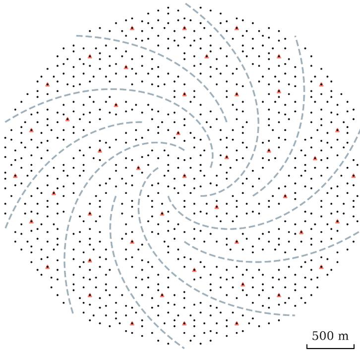
**Fig. 2:** Geometry layout of the TRIDENT array. The pattern follows a Penrose tiling distribution. Each black dot represents a string of length  $\sim 0.7$  km, while the dashed lines mark the paths for underwater maintenance robots.
