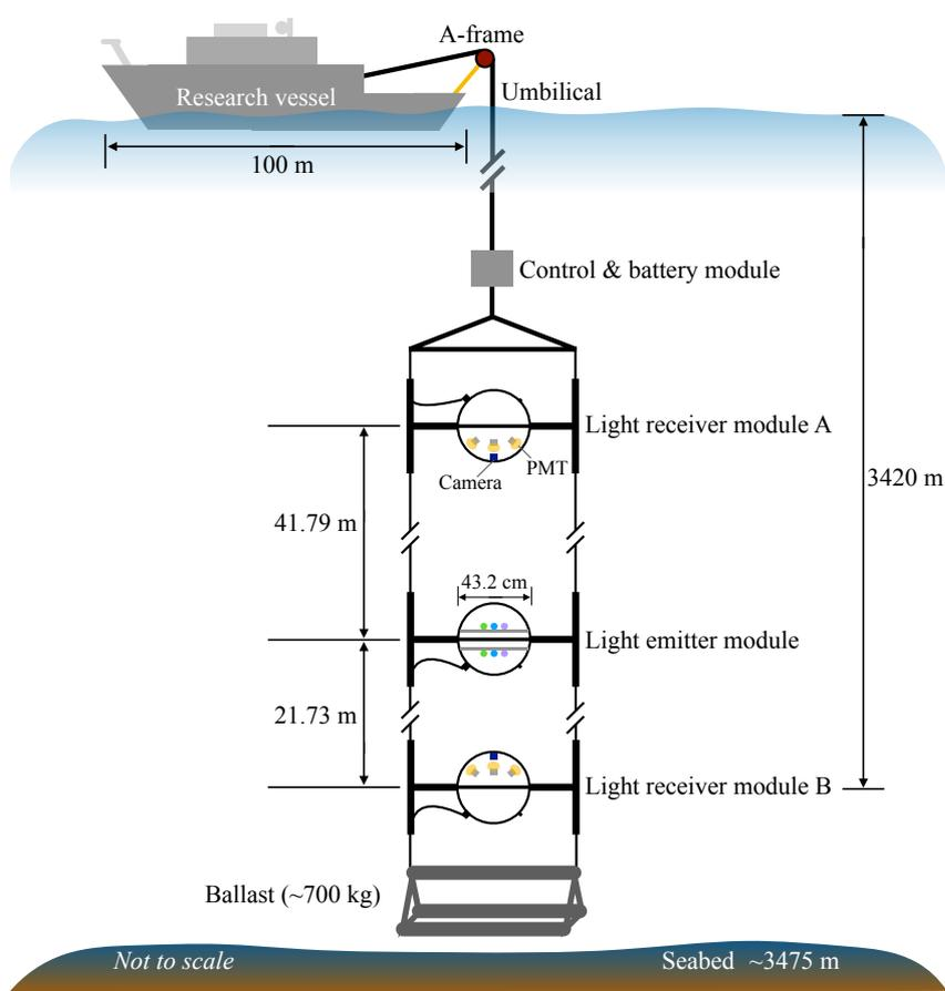
**Extended Data Fig. 4:** The apparatus was deployed to a depth of 3420 m by the umbilical cable from a research vessel. A light emitter module is placed in the middle. Light receiver module A and B are placed on the top and bottom at distances of  $41.79 \pm 0.04$  m and  $21.73 \pm 0.02$  m respectively. Each module is connected to the control and battery module via a composite optical-electric cable for data communications and power supply. This figure is not to scale.
