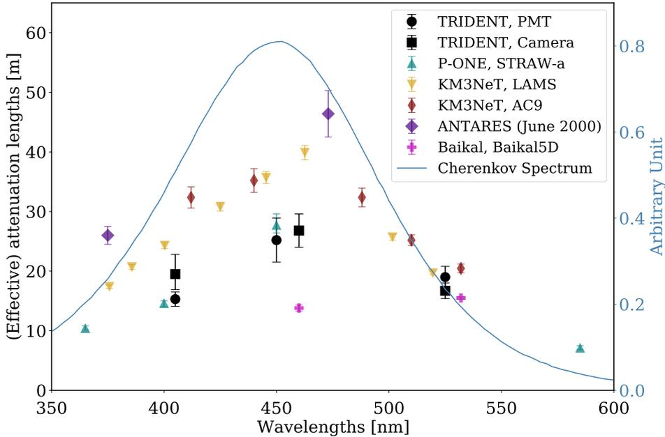
**Fig. 1:** Effective attenuation lengths measured by two independent optical systems, the PMT (black circle) and camera (black square) in T-REX for three wavelengths (405 nm, 450/460 nm, 525 nm). Error bars reflect both statistical and systematic uncertainties. Measurements from KM3NeT [32, 33], P-ONE [34], ANTARES [31], and Baikal-GVD [35] are shown for comparison. Also shown is the observed Cherenkov spectrum from simulation, in which the optical properties measured by T-REX are implemented.
