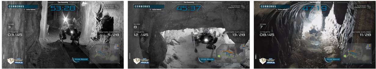
(a) Locomotion challenges front camera (1) planning fails (2) trigger reset (3) replan path
