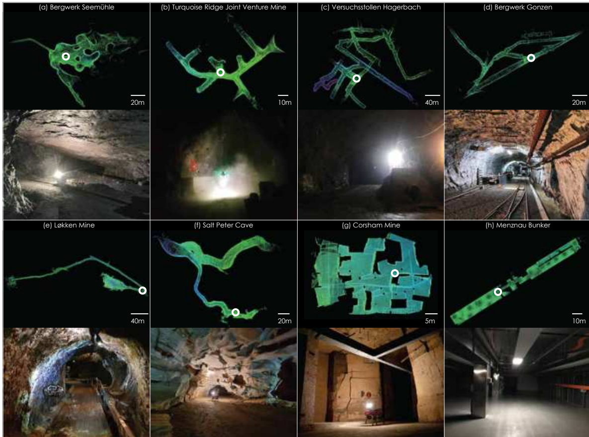
Figure 23: A subset of different underground environments used during the “deployment” phase of field-tests during our participation throughout the SubT Challenge. The first and third rows represent a top-down orthographic view of the reconstructed pointcloud maps of the environments while the second and fourth rows capture a third-person view in these environments. The locations of the image captures are presented in the corresponding maps by a white hollow circle. The challenges presented by each of the environments are discussed in section 4.1.2
