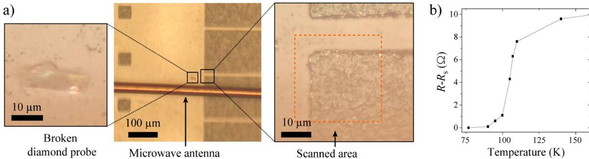
**Fig. S3 | TBCCO sample characteristics.** (a) White light microscope images of the sample also showing the antenna and a broken diamond probe. The dark (white) patches are the superconductor (TBCCO) and the bare substrate (LAO). (b) Resistance of a  $5 \times 5 \text{ mm}^2$  measured with two leads around the transition temperature.
