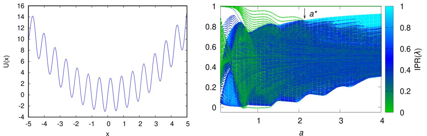
FIG. 17. (left panel) Example of a potential with many local minima given by Eq. (F2). (right panel) Monte Carlo relaxation eigenspectrum for this potential with a flat jump distribution as in Fig. 1 from the main text. The box  $(-5, 5)$  was discretized in  $10^3$  sites.
