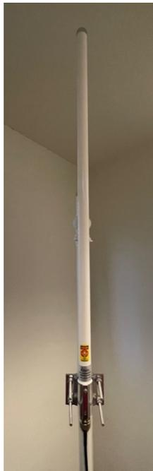
Fig. 12. Altelix Omni-directional 2.4 GHz antenna.
