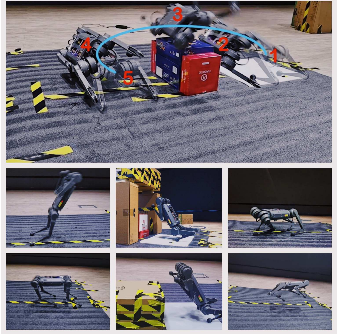
Fig. 1: Applied the proposed method on an open source Mini Cheetah with variety of jumping motion (e.g., front/rear/left/right jumping, yaw-spin jumping, left/right/front/back flipping, jumping with obstacles).
