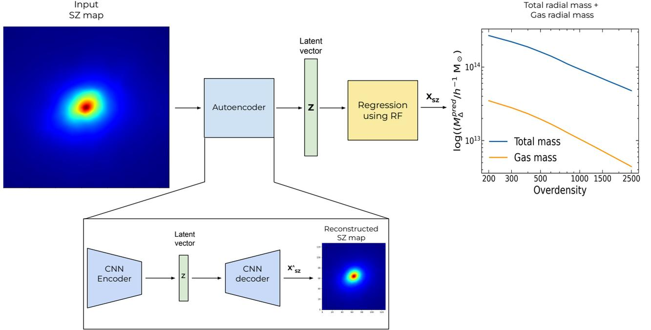
**Figure 2.** The 3D radial mass profile inference architecture using the autoencoder plus the random forest. The autoencoder encrypts the input SZ map in a latent vector. The latter is then used as input for the RF regressor.
