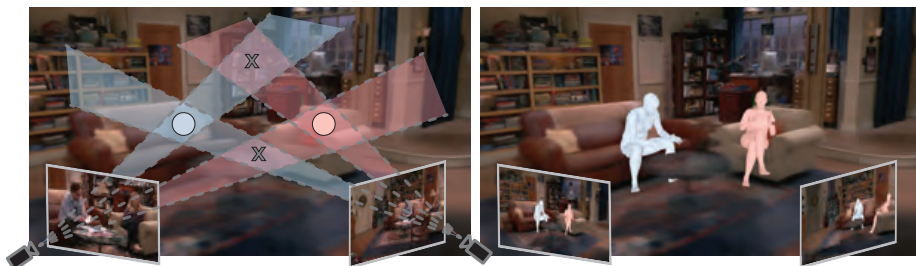
Fig. 5. Calibrated cameras for scale estimation and identity association. Given calibrated cameras, we can use frames at a shot change to solve for the actors’ pose, location, relative scale and association. The four overlapping regions (left) indicate possible locations triangulated by the cameras. Circles indicate correct matches after Hungarian matching. Reconstructed humans are visualized in a NeRF (right).
