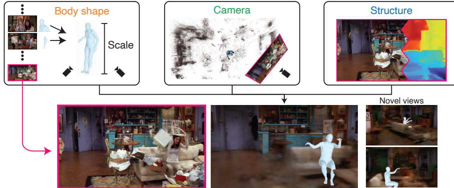
Fig. 6. Contextual monocular human reconstruction. For an input frame, we can leverage (a) the body shape (scale) of the person from a neighboring shot change, (b) the camera registration, and (c) the static structure of the environment. This enables monocular reconstruction of the person in context with their environment.
