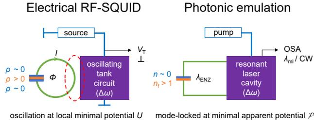
**Figure 1** The schemes of the electric RF-SQUID and its photonic counterpart. Note that in the dispersive mode of the operation of the electric SQUID, the resistance actually remains equal to zero in all components of the superconducting loop due to quantum tunneling.
