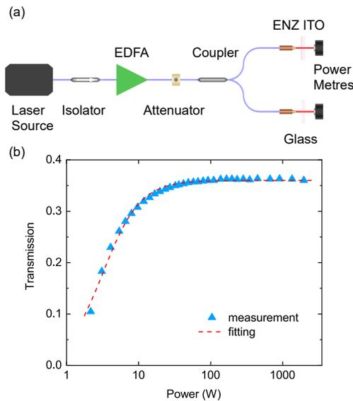
**Figure S3.** Nonlinear saturable absorption measurement. a) The experimental setup; b) The measured results. The triangles denote the data points, and the dashed line represent the fitting curve.
