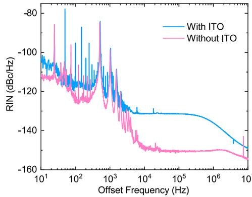
**Figure S2.** Relative intensity noise with and without ENZ ITO.
