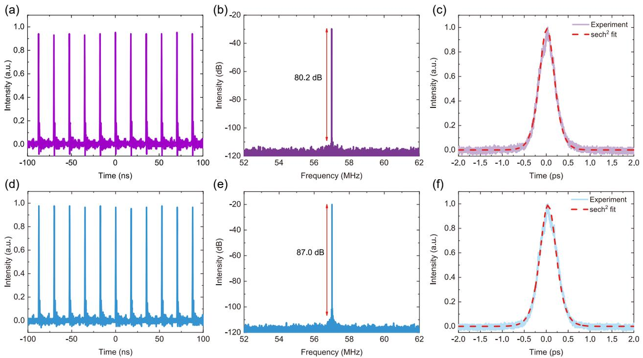
**Figure S1.** Temporal characteristics of the laser output with and without ENZ ITO nanolayer. Temporal profiles with ITO are in the top row, and those without ITO are in the bottom.
