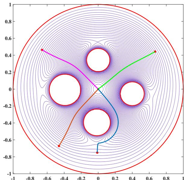
Fig. 2. Trajectories of the kinematic mobile robot (5) under the control law (6) for different initial points in the conformal sphere world.
