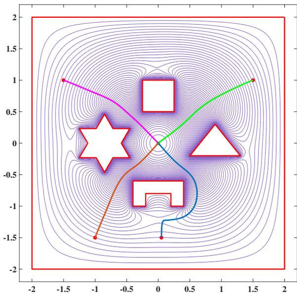
Fig. 1. Trajectories of the kinematic mobile robot (5) under the control law (6) for different initial points in a 2-dimensional polygonal workspace
