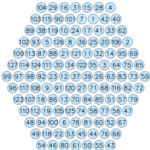
Fig. 3. The schematic view of KOOLS-IFU with fiber ID.
