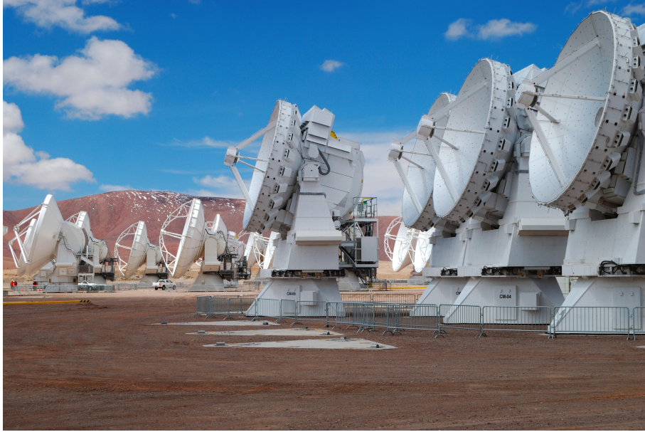
Figure 1. ALMA is an array composed of 50 \times 12 m movable antennas (left background,), 12 \times 7 m fixed antennas (right foreground), and 4 \times 12 m total power antennas.
