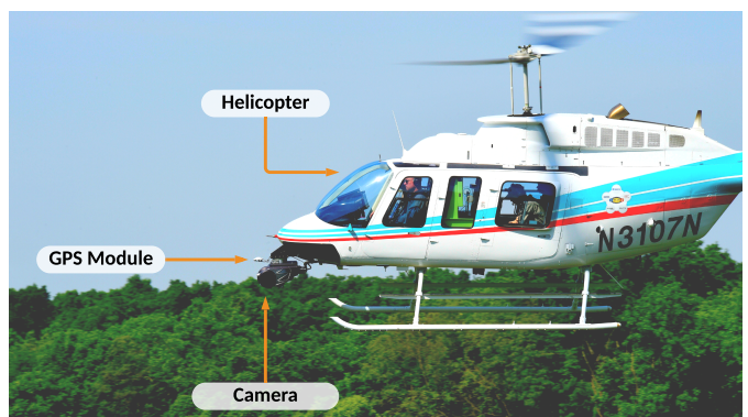
Fig. 7. Helicopter platform. A helicopter equipped with a GPS and a downward-facing pinhole camera is used to collected the 150km long trajectory for localization.
