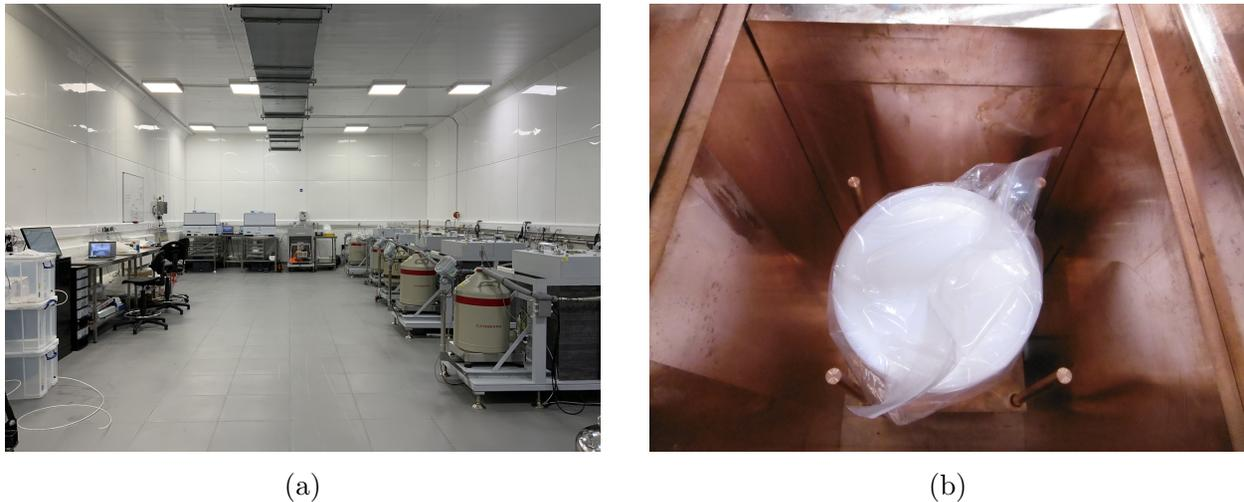
Fig. 3: (a) The BUGS Facility at Boulby Underground Laboratory and (b) a 5 kg  $\text{Gd}_2(\text{SO}_4)_3 \cdot 8\text{H}_2\text{O}$  sample on Merrybent detector.
