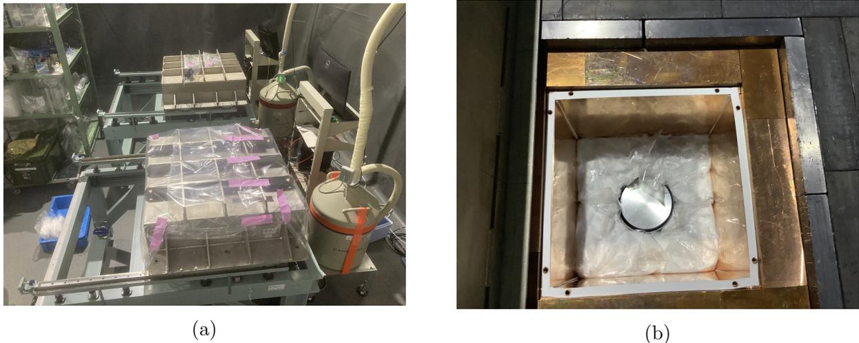
Fig. 5: (a) Ge detectors in Lab-C at Kamioka Observatory, (b) Kamioka Lab-C Ge detector with 10 kg of  $\text{Gd}_2(\text{SO}_4)_3 \cdot 8\text{H}_2\text{O}$  in EVOH bags loaded for measurement.
