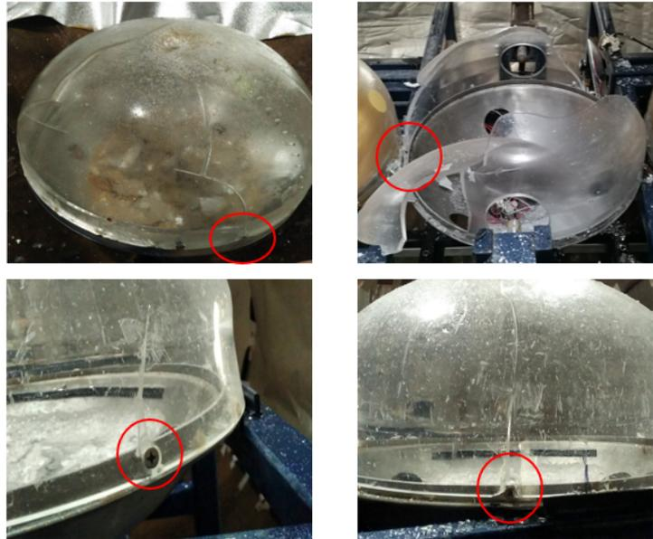
Figure 13: Cracks generated on the acrylic cover in the underwater experiments, all starting from the connection points between top and bottom covers.
