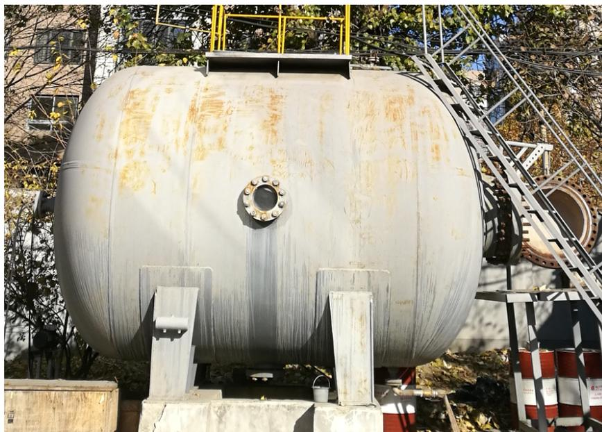
Figure 8: Pressure tank made of steel used for the underwater test. The inner volume is  $35 \text{ m}^3$ . Four acrylic windows on the wall of the tank are used for the high-speed camera or the light.
