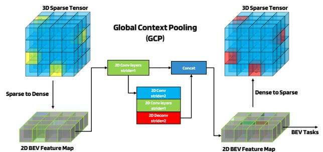
Figure 3: **Illustration of the Global Context Pooling (GCP) module.** 3D sparse tensor is projected to a 2D BEV feature map. Two levels of 2D BEV feature maps are concatenated and then converted back to a 3D sparse tensor, which serves as the input to the BEV task heads.
