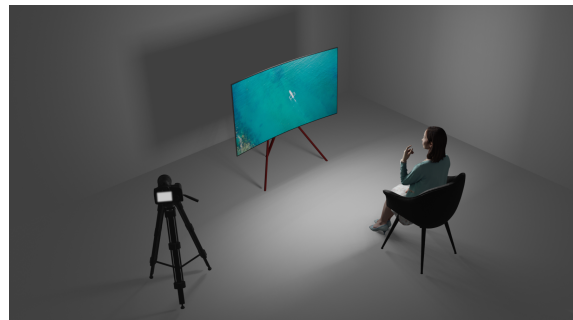
Figure 1: Consider an illustrative scenario where an individual sits across a TV screen in a given room, and suppose that the light reflected by the individual creates a shadow of the screen cast on a blank wall. We demonstrate that such shadows have a potential to leak biometric information in various scene configurations.
