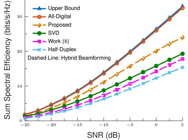
Fig. 5: Sum spectral efficiency results: Performance comparison between the proposed algorithm with the related works as well as the benchmarking tools.
