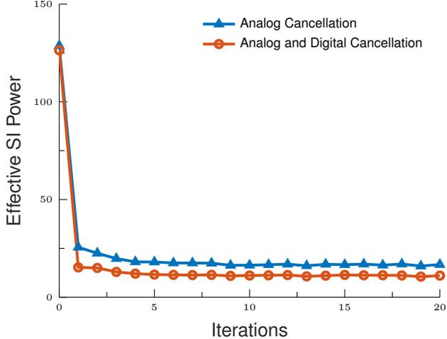
Fig. 4: Convergence of the effective SI power function implemented in analog ( $\mathcal{J}$ ) defined in the objective function (23) and hybrid analog/digital for the proposed hybrid beamforming algorithm 1. The plot is produced with SNR = 0 dB and SI power  $\rho_s = 15$  dB.
