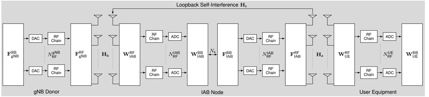
Fig. 2: Basic abstraction of the hybrid analog/digital architecture of the full-duplex integrated access and backhaul system. The backhaul channel is between the gNB donor and IAB node, and the access channel is between the IAB node and the user equipment.
