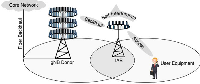
Fig. 1: Full-duplex integrated access and backhaul (IAB) for a single-user case. The gNB donor, linked to the core network by fiber backhaul, communicates with the IAB node through wireless backhaul. The user equipment is served by the IAB node through the wireless access link. Simultaneous transmission and reception of the IAB node over the same time/frequency resources blocks incurs loopback self-interference.
