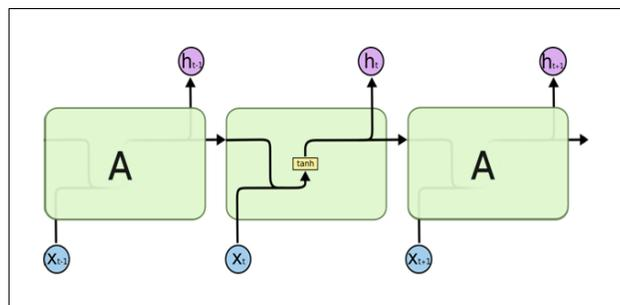
Figure 2: The repeating module in a standard RNN contains a single layer.
