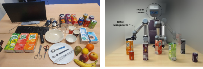
Fig. 4: A subset of the object catalogue included in the HOTS dataset (left) and an image of our real robot setup from the opposite perspective (right).
