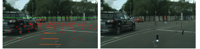
Figure 4: Left: Anchor points distributed along the road surface. We place obstacles at a random subset of anchor points. Right: Frame with injected obstacles.
