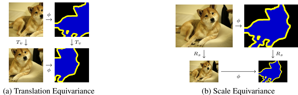
Figure 1: Example of equivariance in the cases of translation and scaling. In this case, \phi is an ideal operator that computes the semantic segmentation of images. The operators T_v and R_s are, respectively, a translation and a re-scaling.
