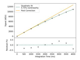
Figure 4: Mean signal of a 200 by 200 pixel area against increasing integration times. Residual plot is the deviation from the linear regression as a percentage.
