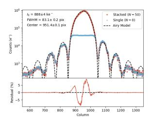
Figure 8: Reduced line profiles of first Airy reflection using HDR and standard readout modes. HDR data is fit to an Airy to model allow for parameter extraction. The standard scheme clips at pixel saturation. Residuals of HDR line profile deviate beyond error bars imposed by Poisson statistics, signifying that deviations in fit are from optical interference and misalignment.
