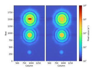
Figure 7: A comparison of the three reflected Airy patterns using the HDR and standard readout schemes. Left is an image of the Airy pattern using the HDR scheme, right is the same pattern with the standard scheme. The majority of pixels in the first order ring of the primary and secondary reflection are saturated at 25 ke<sup>-</sup>. By contrast, pixels up to 937 ke<sup>-</sup> are recorded in the linear regime for the HDR region.
