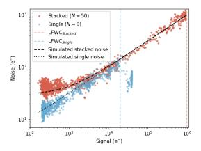
Figure 10: First reflection line profile noise (estimated with  $9 \times 3$  window) vs window mean for HDR, standard scheme and expected shot noise. The HDR scheme is in a read noise dominated regime at low signals ( $<3~{\rm ke^-}$ ) whereas the standard scheme remains in a shot noise regime. Noise for the HDR scheme follows Poisson statistics until peak intensity at 984 ke<sup>-</sup>, whereas the standard readout hits saturation.
