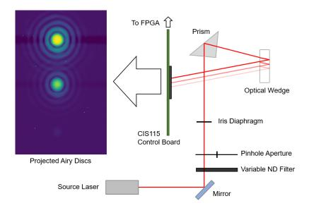
Figure 3: Optical setup used. Laser source is a Thorlabs CPS532-C2, ND filter a Thorlabs NDC-50C-4, mirror, Thorlabs PHWM16 pinhole, 45 degree prism, a Thorlabs WW41050-A optical wedge and the CIS115 board. The optics are used to project the three Airy Discs shown in the top left
