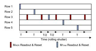
Figure 1: Simplified row-wise timing diagram in rolling shutter operation. In this example for N=5, row three is read out six times in one integration whilst the other four rows just once. Integration occurs in the white regions with readout and reset samples in the blue for the standard readout and in red for the HDR readout.
