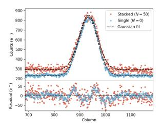
Figure 9: Reduced line profiles of third Airy reflection using HDR and standard readout modes. The HDR scheme shows both higher background noise (34 e $^-$  vs 15 e $^-$ ) and background offset (295 e $^-$  vs 234 e $^-$ ) compared to the standard readout. Both models are fit to a Gaussian as opposed to an Airy disc as the noise washes out all but the first order.
