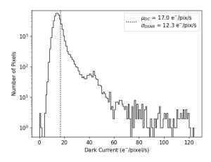
Figure 5: Dark current distribution for 200 by 200 pixels, bin width of 1 e<sup>-</sup>/pixel/s. Dotted line represents the average dark current. The distribution has a component which follows the normal distribution, as well as a tail of pixels with high dark current. Measurements were taken at 294 K.
