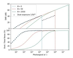
Figure 2: Noise performance at varying photosignals for the HDR extension scheme described in this paper. N is the number of additional row signal and reset samples per integration.
