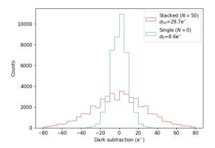
Figure 6: Noise distribution of dark frames for rows in the HDR scheme (red) and standard scheme (blue), bin width of 5 e<sup>-</sup>. Noise increases from 8.6e to 29.7e in the N=50 regions due to the read noise adding in quadrature.
