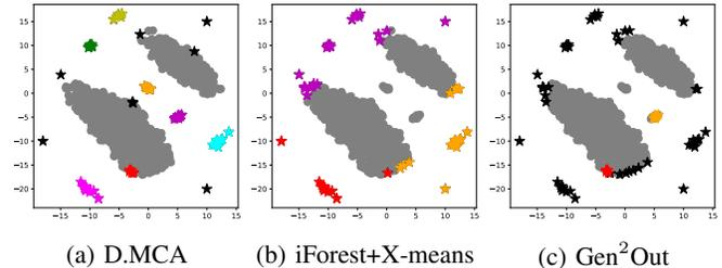
Fig. 1: Example dataset with two inlier modalities (gray dots), with scattered and clustered outliers. (a) Proposed D.MCA effectively flags the outliers (stars) and also explicitly assigns to micro-clusters (colored differently). (b) Two-stage solutions, detection+post hoc clustering, are not as effective. (c) SOTA baseline underperforms, often missing interior outliers.
