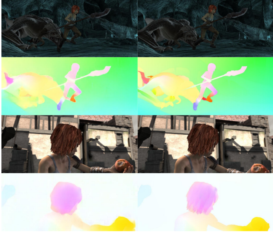
Figure 12: Qualitative visualization of the estimated flow on some examples from the MPI-Sintel training set, unseen during training. First and third rows: input image pair, second and fourth row: predicted ( left ) and ground-truth ( right ) flows.
