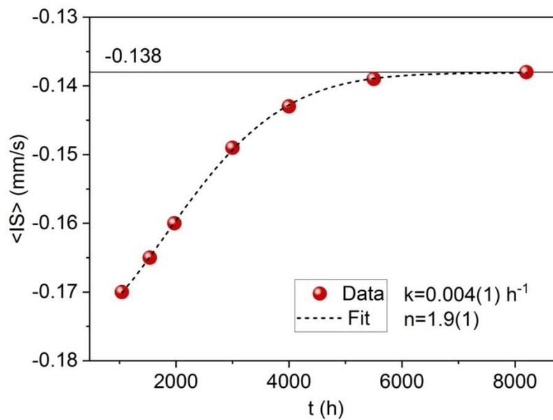
Fig. 12 Time dependence of the average isomer shift,  $\langle IS \rangle$ , for the final stage of annealing. The solid line stands for the best-fit of the data to the JMAK-equation. The
