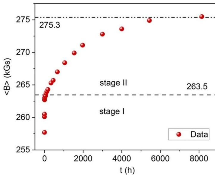
Fig. 3 Average hyperfine field,  $\langle B \rangle$ , vs. annealing time,  $t$ . Two stages of the decomposition process are marked – see also Fig. 4. Maximum values of  $\langle B \rangle$  in each of the stages are denoted by horizontal lines and correspondingly labelled.
