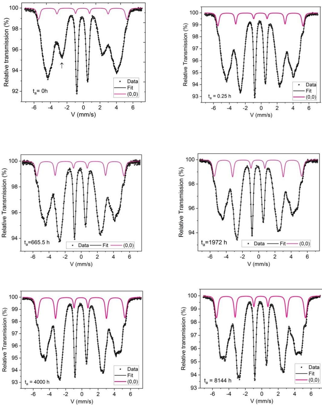
Fig. 1 Examples of Mössbauer spectra recorded on the  $\text{Fe}_{73.7}\text{Cr}_{26.3}$  sample annealed at  $585^\circ\text{C}$  for different periods,  $t_a$ , as indicated for each spectrum.
