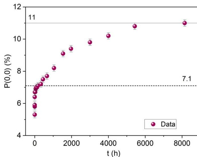
Fig. 13 Dependence of the  $P(0,0)$  probability on the annealing time,  $t$ , for the whole range of annealing viz.  $0 \leq t \leq 8144$  h. The line at  $P(0,0) = 7.1$  % stands for the maximum value of  $P(0,0)$  achieved in the first stage of transformation. The line at
