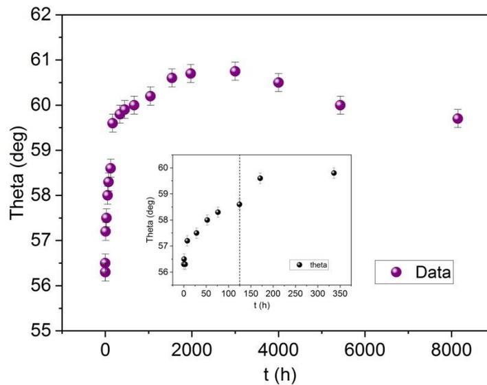
Fig. 16 Dependence of theta on the annealing time,  $t$ , for the whole range of annealing viz.  $0 \leq t \leq 8144$  h. The inset shows the behavior of theta within the first ~350 hours of annealing.
