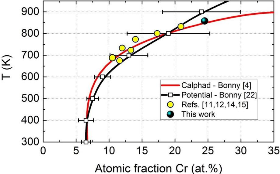
Fig. 8 Comparison between two theoretical predictions depicting the miscibility gap in the Fe-Cr system [24] and experimental data obtained with the Mössbauer spectroscopy. The size of the symbols is comparable with the error in the Cr content..
