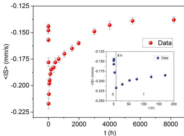
Fig. 10 Annealing time dependence of the average isomer shift,  $\langle IS \rangle$ . The inset shows the  $\langle IS \rangle(t)$  behavior within the first 170 hours of the annealing.
