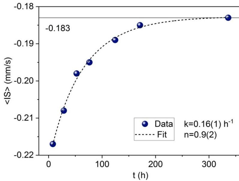
Fig. 11 Annealing time dependence of the average isomer shift,  $\langle IS \rangle$ , for the first 335 hours of annealing. The dashed line stands for the best-fit of the data to the JMAK-equation. The best-fit parameters are displayed. The value of  $\langle IS \rangle$  -0.183 mm/s in saturation is indicated.
