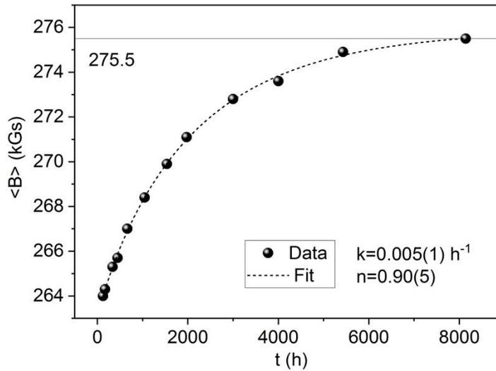
Fig. 6. Average hyperfine field,  $\langle B \rangle$ , as a function of the annealing time,  $t$ , for the second stage of the transformation process. The best-fit of the data to eq.(1) is indicated by the dashed line. Values of the kinetic parameters  $k$  and  $n$  as well as that of  $\langle B \rangle_{max}$  are shown.
