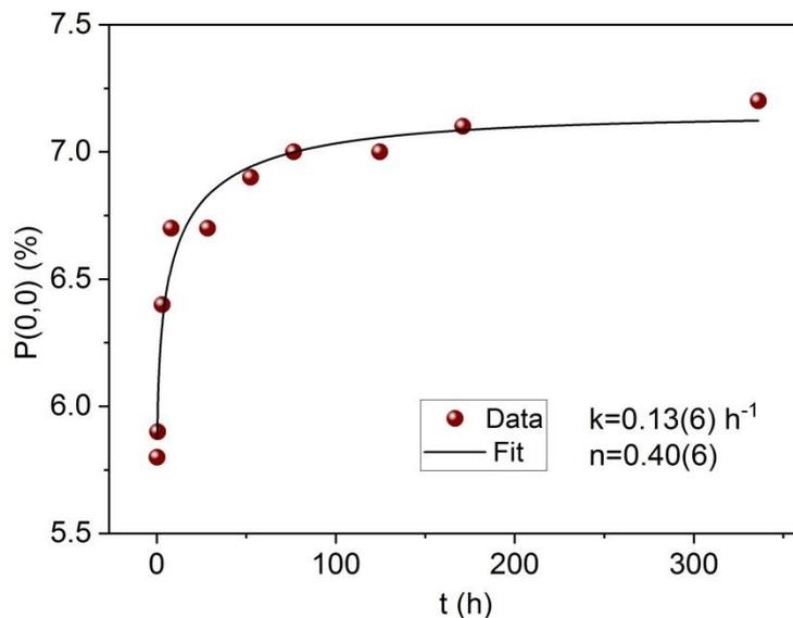
Fig. 14 Dependence of the  $P(0,0)$  probability on the annealing time,  $t$ , for the first stage viz.  $0 \leq t \leq \sim 350$  h. The line represents the best-fit of the data to the JMAK-like equation. The kinetics parameters,  $k$  and  $n$  are displayed.
