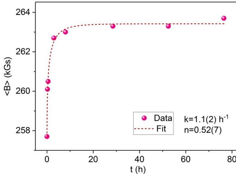
Figure 5. Average hyperfine field,  $\langle B \rangle$ , as a function of the annealing time,  $t$ , for the first stage of the transformation process. The best-fit of the data to eq.(1) is indicated by the dashed line. Values of the kinetic parameters  $k$  and  $n$  are displayed.
