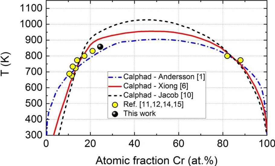
Fig. 7 Comparison between three theoretical Calphad-based predictions concerning the full MG adopted from [10] and our experimental data obtained with the Mössbauer spectroscopy. The size of the corresponding symbols is comparable with the experimental error in the Cr content.
