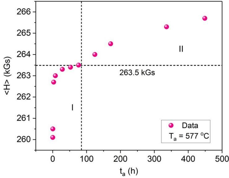
Fig. 4 Average hyperfine field,  $\langle B \rangle$ , vs. annealing time,  $t$ , for the first ~450 hours of annealing. A vertical dashed line indicates a transition between the first and the second stage of a transformation process. The horizontal dashed line marks the maximum value of  $\langle B \rangle$  in the first stage.
