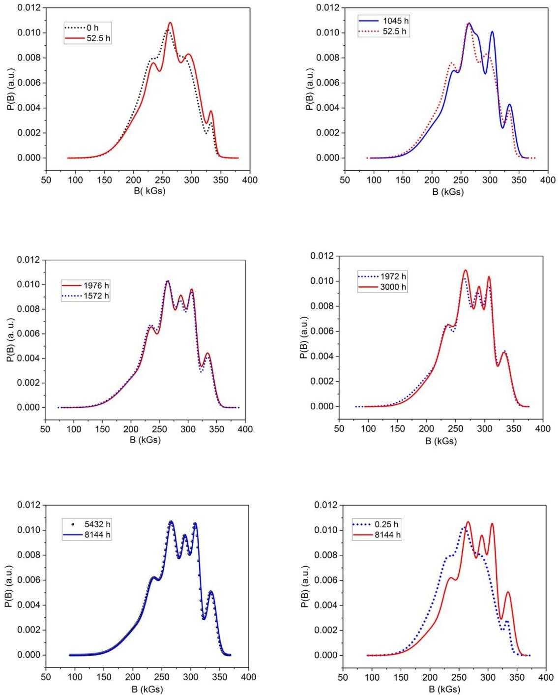
Fig. 2 Comparison between the  $P(B)$ -curves derived from the spectra annealed for different periods between 0 h and 8144 h. Notice that there is no more difference between the  $P(B)$ -curves for 5432 h and 8144 h.
