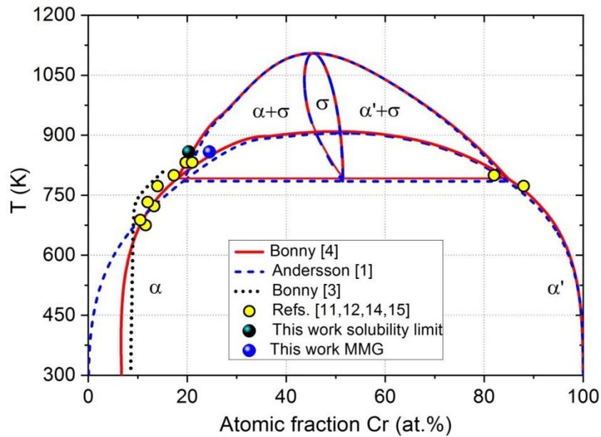
Fig.9 Relation between experimental data obtained with the Mössbauer spectroscopy and the calculated phase diagram of the Fe-Cr system adopted from [4]. Size of the symbols corresponds to the uncertainty in determination of the Cr content.
