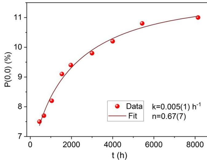
Fig. 15 Dependence of the  $P(0,0)$  probability on the annealing time,  $t$ , for the annealing time between  $\sim 350$ h and 8144h. The line represents the best-fit of the data to the JMAK-like equation. The kinetics parameters,  $k$  and  $n$  are displayed.
