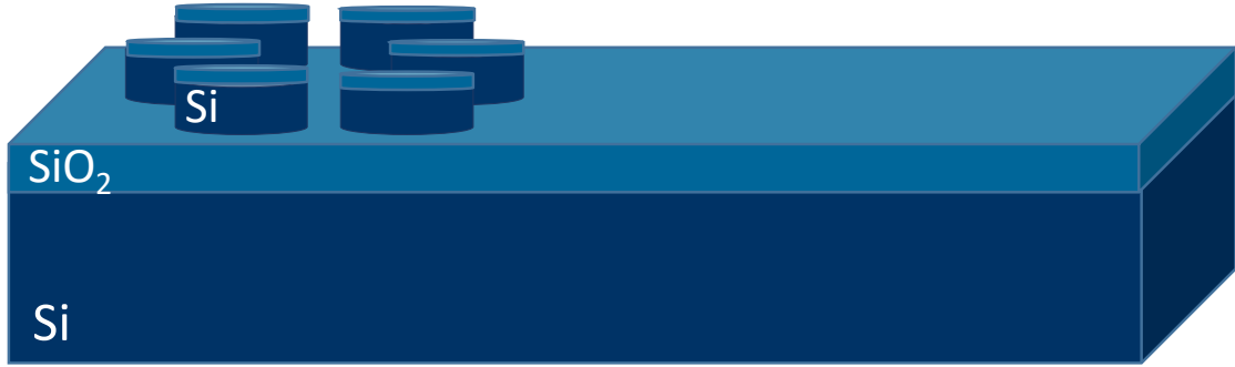
FIG. 12: Side view of the substrate with MoSe 2 on top. From top to bottom the first SiO 2 layer is 30 nm of height, Si pillars are 95 nm + SiO 2 30 nm, SiO 2 layer is 145 nm thick, everything on a Si substrate.
