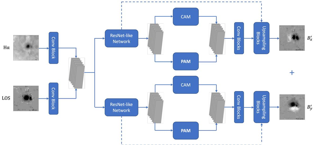
**Figure 2.** Illustration of the architecture of the MagNet model. The model takes as input a pair of coaligned AR patches of H $\alpha$  image and HMI/MDI LOS magnetogram, and generates as output the pair of AR patches of  $B'_x$  and  $B'_y$  that correspond to the input data. See text for details of the model architecture.
