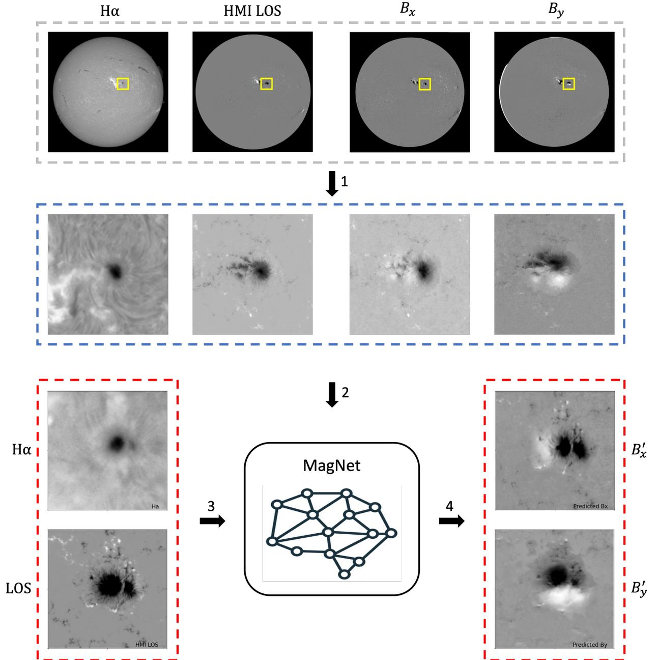
**Figure 1.** The workflow of MagNet. During training, we coalign and crop AR patches of  $256 \times 256$  pixels from four full disk images (step 1) and use the coaligned AR patches to train the MagNet model (step 2). During testing/prediction, a pair of coaligned AR patches of H $\alpha$  image and HMI/MDI LOS magnetogram is fed to the trained Magnet model (step 3), which generates the pair of AR patches of  $B'_x$  and  $B'_y$  that correspond to the input test data (step 4).
