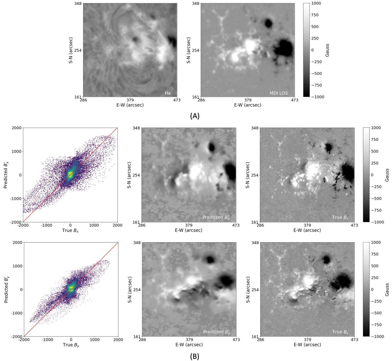
**Figure 6.** Comparison between MagNet-generated  $B'_x$ ,  $B'_y$  and true  $B_x$ ,  $B_y$  based on BBSO H $\alpha$  and MDI LOS data of AR 11117 on 2010 October 27 22:24:00 UT. (A) The H $\alpha$  and MDI LOS data inputted to MagNet. (B) The output results from MagNet.
