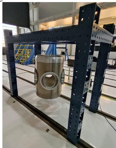
Fig. 11. Kick-Stage ESPA tower under natural frequency assessment
