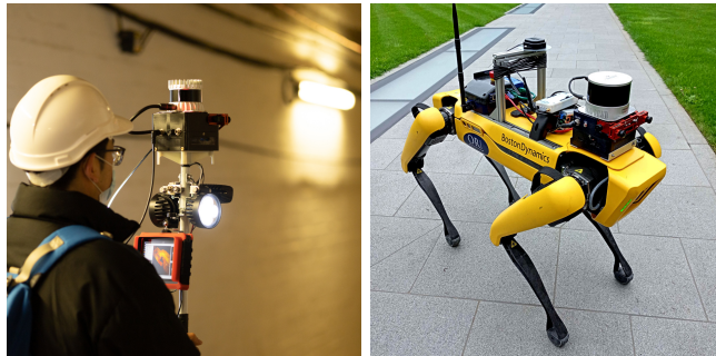
Fig. 1. Two of the platforms used in this work. Left: handheld device including a SevenSense AlphaSense visual-inertial sensor. Right: the same device mounted on a Boston Dynamics Spot quadruped. An IMU bias model from a neural network trained on handheld data was used to infer the biases on the Spot dataset without any retraining — despite the significantly different motion pattern. The lidar was not used in these experiments.
