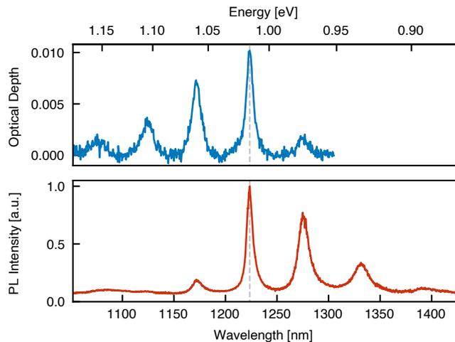
FIG. 1. Absorption and PL spectroscopy. Room temperature absorption (top) and PL (bottom) spectra at 285 K for sample 1 with narrow peaks evenly spaced by approximately 42 meV. The two spectra display a clear mirror symmetry, with the mirror axis being the brightest line at 1224 nm. The grey dashed line shows the axis of symmetry as a guide to the eye. The thickness of the sample is 0.66 mm.
