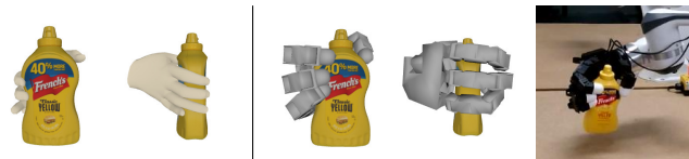
Fig. 5. Real-world experiments. Left : input human demonstration. Middle : corresponding Allegro grasp prediction. Right : execution.
