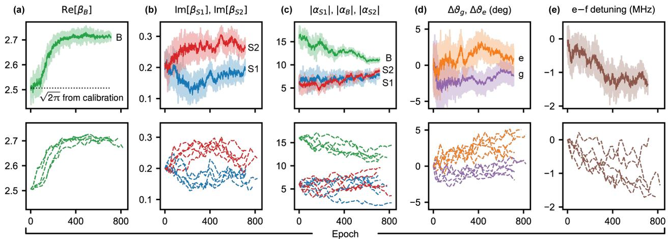
FIG. S14. **Evolution of QEC circuit parameters during the training.** Top row: example from one particular training run. The shaded region bounds the minimal and maximal sampled parameter values. Solid lines indicate the mean. Bottom row: evolution of the mean parameter values in several independent training runs performed during a two-day period, showcasing the reproducibility of the training results.
