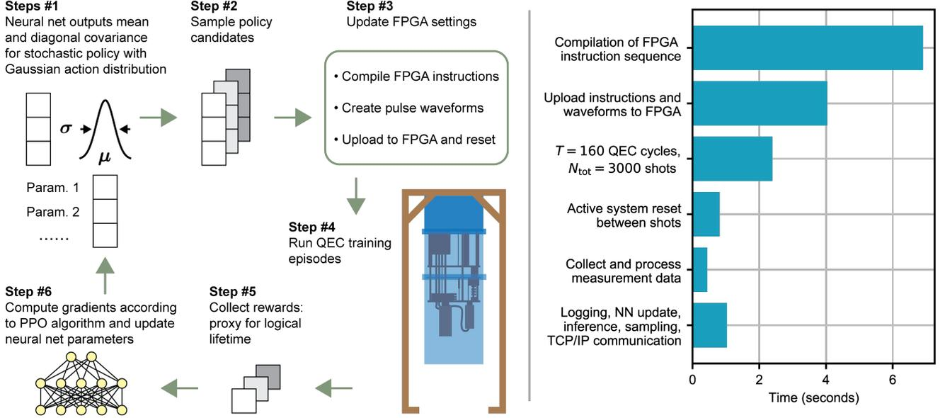
FIG. S11. **Reinforcement learning.** (a) Experimental training loop. (b) Training time budget per epoch.
