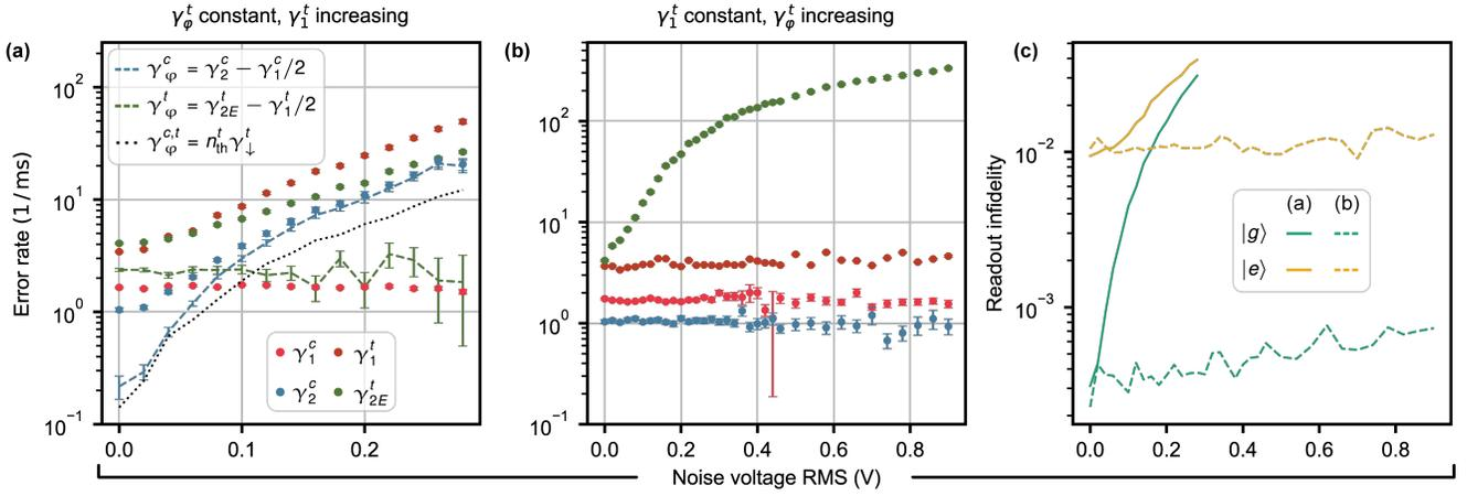
FIG. S23. **Noise verification experiments.** (a) Component error rates as a function of the root mean square (RMS) voltage of the injected noise (at the generator plane). Here, noise is up-converted to the qubit frequency to increase  $\gamma_1^t$ . (b) Same as in (a), but with the baseband noise that increases  $\gamma_\phi^t$ . (c) Readout infidelity of the transmon  $|g\rangle$  and  $|e\rangle$  states in these two noise injection settings.
