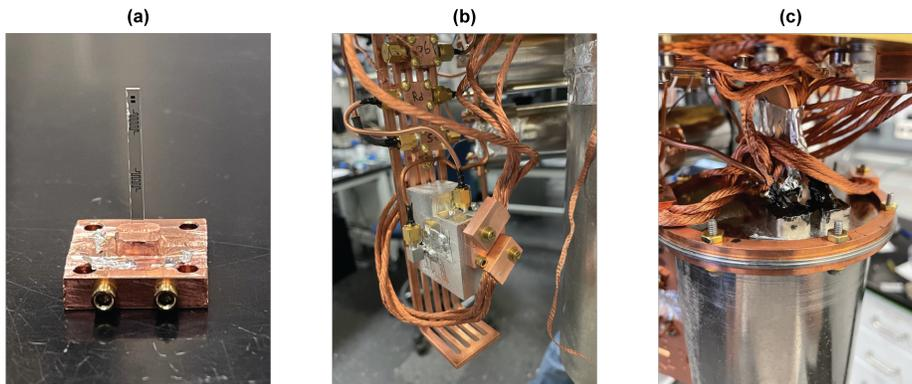
FIG. S1. **Sample assembly.** (a) Clamped ancilla chip. (b) Thermalization. (c) Shielding.
