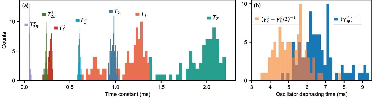
FIG. S7. **Fluctuating error channels.** (a) Histogram of  $T_1$  and  $T_2$  times of the transmon and the oscillator, and logical lifetimes of error-corrected grid states. The histogram is derived from a week-long scan described in Chapter S4 J. (b) Oscillator pure dephasing time extracted from the measured oscillator parameters and predicted from the dispersive coupling model.
