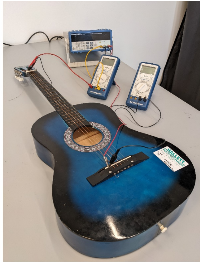
Figure 1: A closed circuit created on a guitar with music wire, a power supply, and two multimeters to measure voltage and current.
