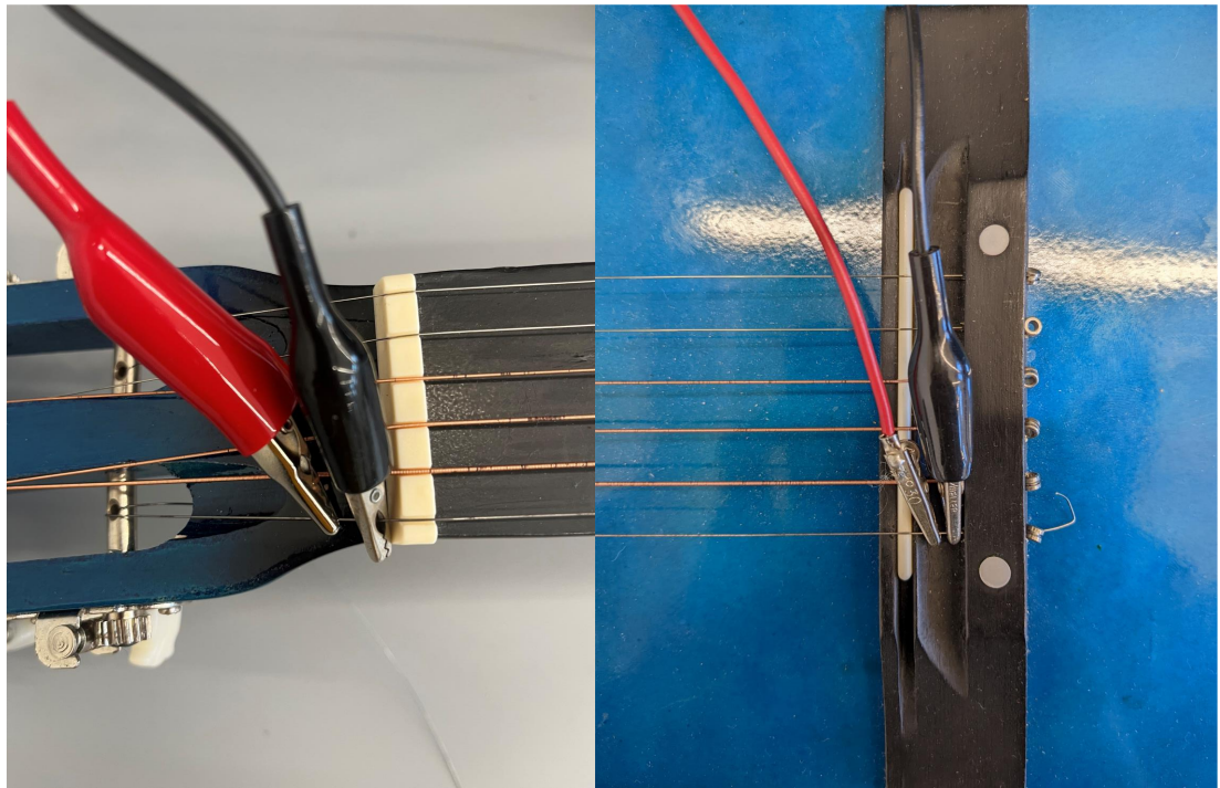
Figure 2: The connection points on both ends of the guitar. All connections are placed above the nut (left) and below the saddle (right) to ensure that the electrical connections do not interfere with the harmonics of the plucked wire.
