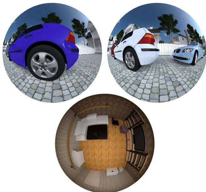
Fig. 1. Example frames of synthetically generated equisolid fisheye video sequences. Top: Street , bottom: Room .
