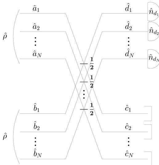
Figure 3. Circuit implementing the measurement of the purity and QCS for a  $N$ -mode state  $\hat{\rho}$ . Here, two identical copies of the state are sent in a stack of 50:50 beam splitters and the photon number statistics is measured in the output modes  $\hat{d}_k$ , with  $k = 1, \dots, N$ .
