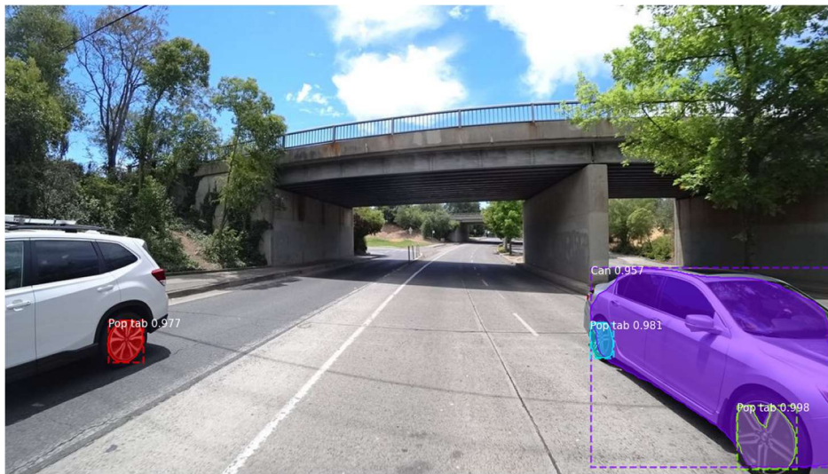
Fig. 7. Cars being recognized as cans with pop tabs for tires by Mask R-CNN. [13]
