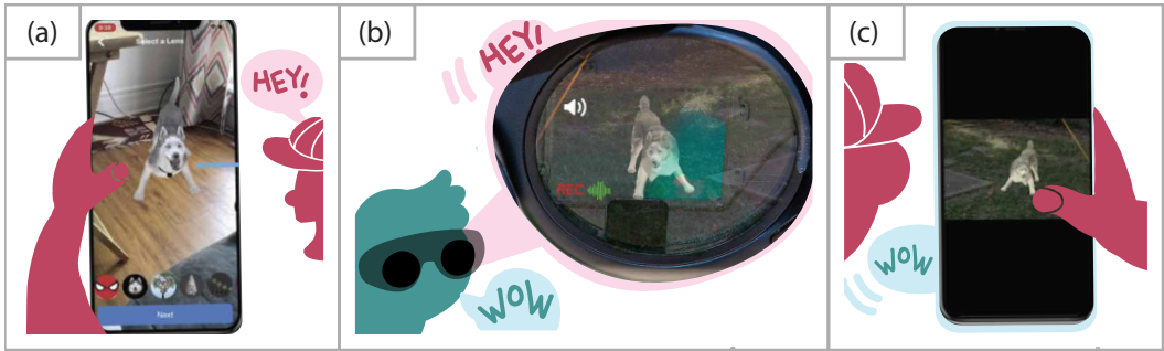
Fig. 1. Overview of ARwand: (a) A smartphone user (sender) sends an AR message (AR content with a voice note) to their friend (recipient) who owns smartglasses. In this case, the AR message is a barking dog accompanied by the sender saying “Hey!” (b) ARwand auto-captures a video of the recipient’s reaction (“Wow!”) while they experience the AR message. The video is sent to the sender once the recipient confirms. (c) The sender views the recipient’s reaction video.
