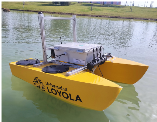
Figure 1: An Autonomous Surface Vehicle used for water resources monitoring system
