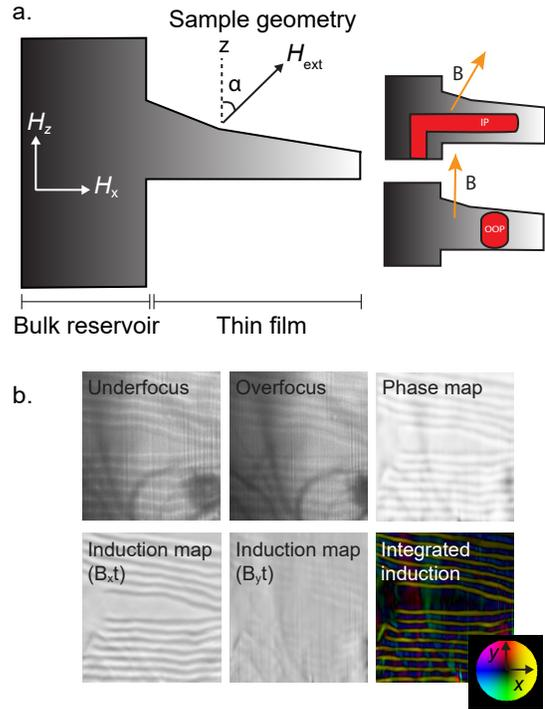
FIG. S1: (a) Schematic of the experimental geometry. The angle,  $\alpha$ , is defined as the angle between the film normal and the applied field. (b) Underfocus and overfocus LTEM image showing the reconstruction of magnetic phase.
